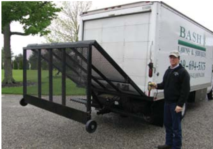
Tim installed a hydraulic cylinder on the box truck for raising and lowering the ramp.
